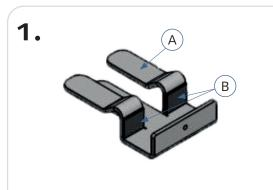
Apply the foam pads [B] to the parts of the soni FIX CLAMP [A] that will rest on the desk/table surface.
